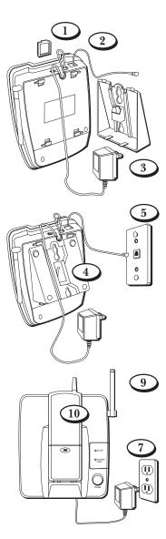
10. Place handset in the base to charge for 12 hours. The CHARGE/PAGE light comes on to indicate that the battery is charging. You must charge the handset battery continuously (without using the phone) for 12 hours when you set up the phone.
